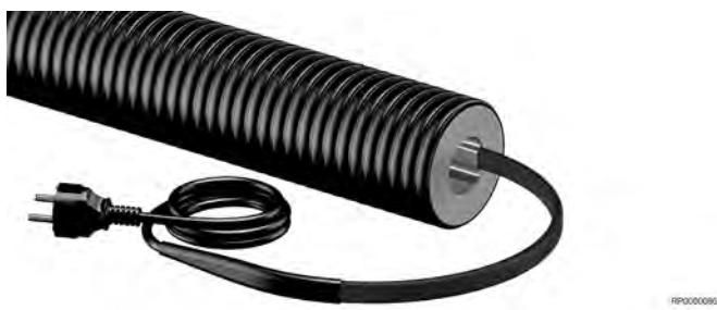
Ecoflex Mantle is an insulated jacket for water pipe inlet. It protects the parts of a water pipe most susceptible to freezing, generally near the building foundation or inside a ventilated floor system. The jacket can be used for new buildings and renovation.
