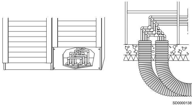
The flexibility of the piping system allows for planning the trenches flexibly and taking the environment into account. When the pipe element is led into the building, the selection of the entry location must take into account the space requirements of the pipe bending radius.
