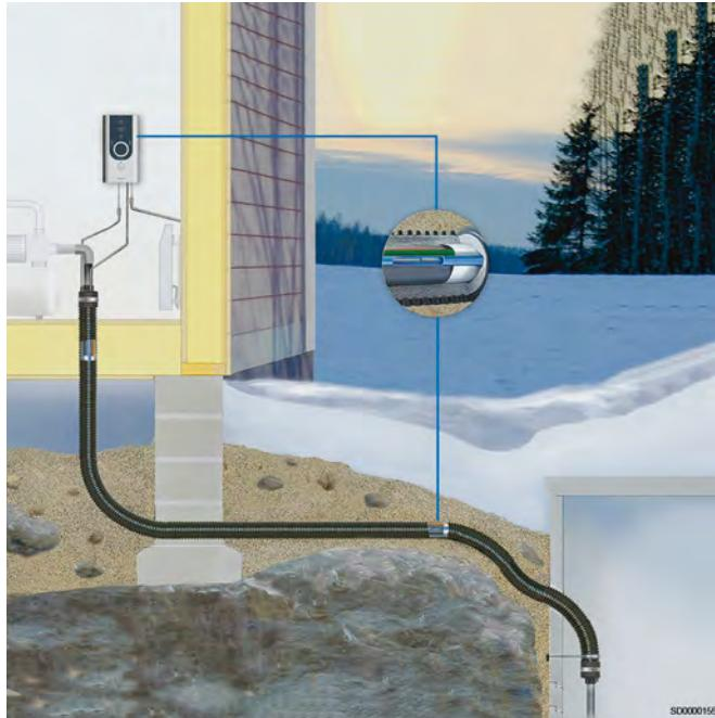
The frost protection cable of the Supra PLUS pipe is self-regulating and thus cannot overheat.
