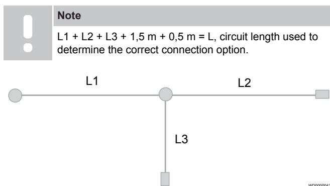
The lengths of the pipes are added up. Add 0,5 m for both connection and termination and 1,5 m for each branching. Also add enough cable to wrap around additional sources of thermal loss (valves, inlets, etc.). In extensive networks, lines should be grouped in suitable connection circuits so that the cable provides the required output per meter W/m (see the heating capacity charts).
