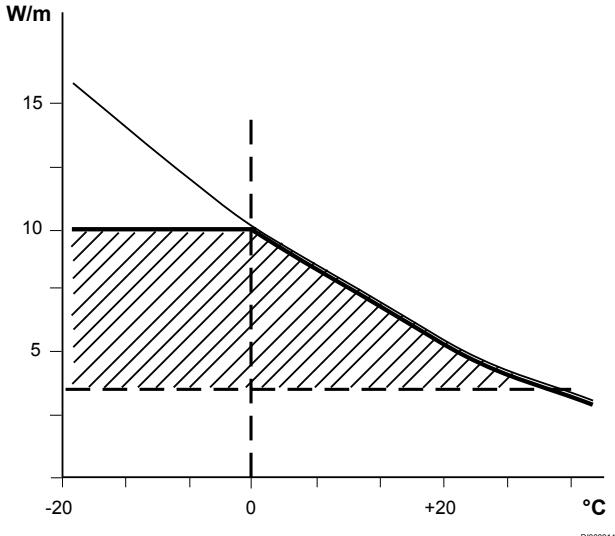
The frost protection cable supplies full power in ice, cold water or in a frozen pipeline. The ruled area in the image shows the input power W/m depending on the outdoor temperature when the frost protection cable is on continuously.
