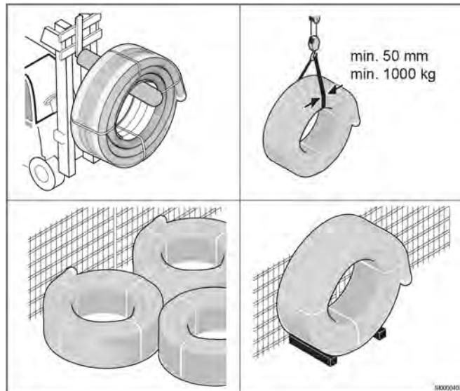
Do not drag the coil across rough surfaces. Ensure that the coil is not squashed and that the pipe is not dented when bent during storage. Store all coils in a horizontal position. Pipe coils and chambers can be stored outside, other components of the system should be stored indoors.
