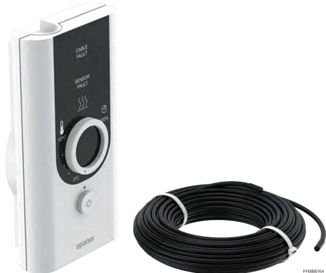
The Uponor Ecoflex Supra PLUS control unit is an electronic regulator designed for controlling the self-regulating frost protection cable of the Supra PLUS pipe. The control unit has two different functions, either a function with a temperature sensor or a fixed timer function.
