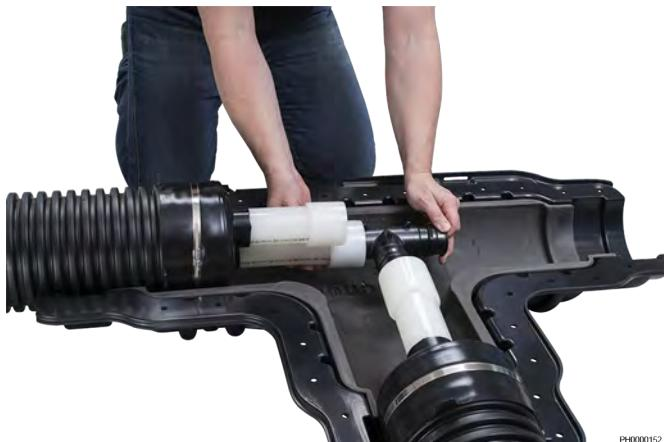
The Uponor Q&E fitting is based on a method where a Uponor PE-Xa pipe is gradually expanded with a Q&E (PEX) ring fitted on the outside, and then allowing it to shrink back onto a fitting nipple. The technique can be used as the Uponor PEX material is capable of shrinking back to almost its original size, even after a very large amount of expansion.
