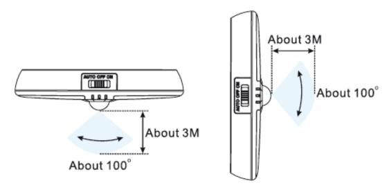
The above measurements are measured at a temperature of 25°C. The sensing range of infrared sensors varies slightly according to temperatures.
